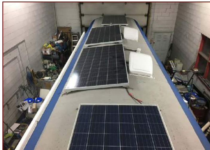
Solar Panels on Opti-Force 1.
